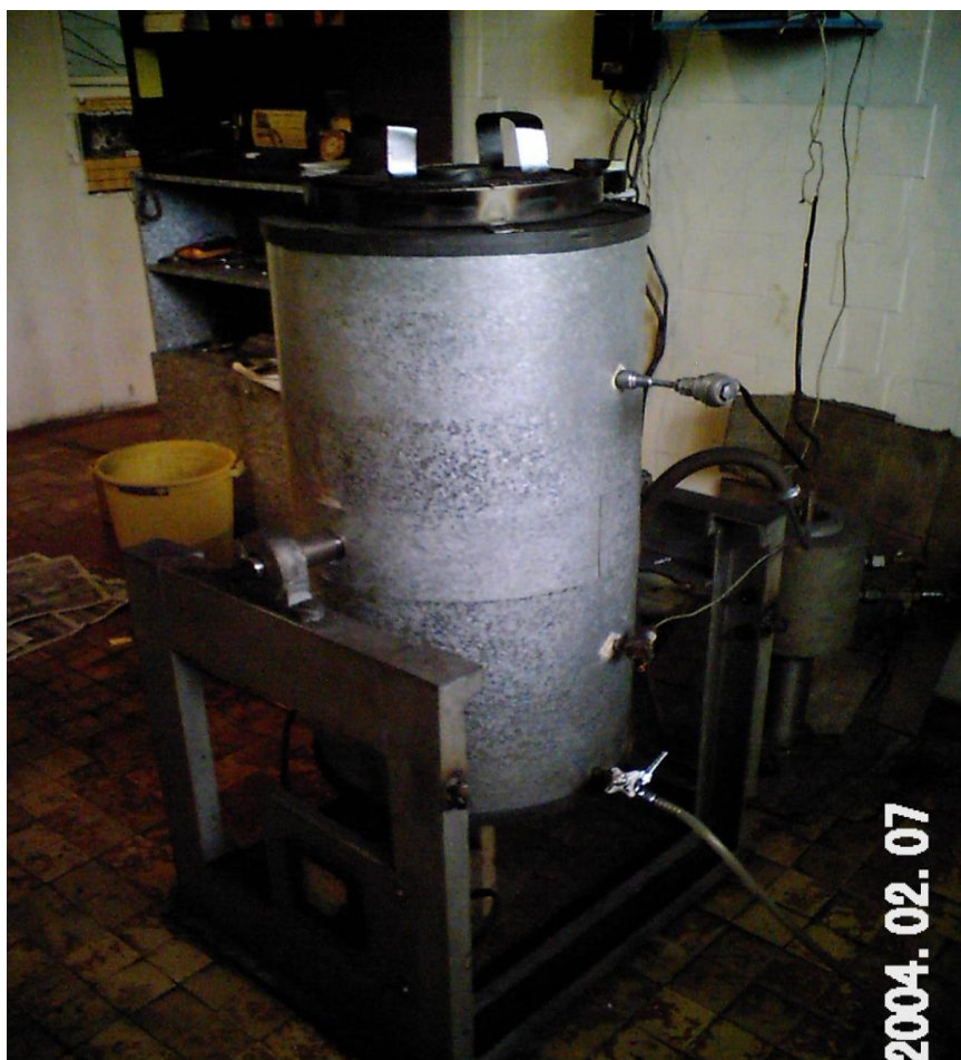
Figure 44 – A photography of the thermal burning and hot steam activation unit
