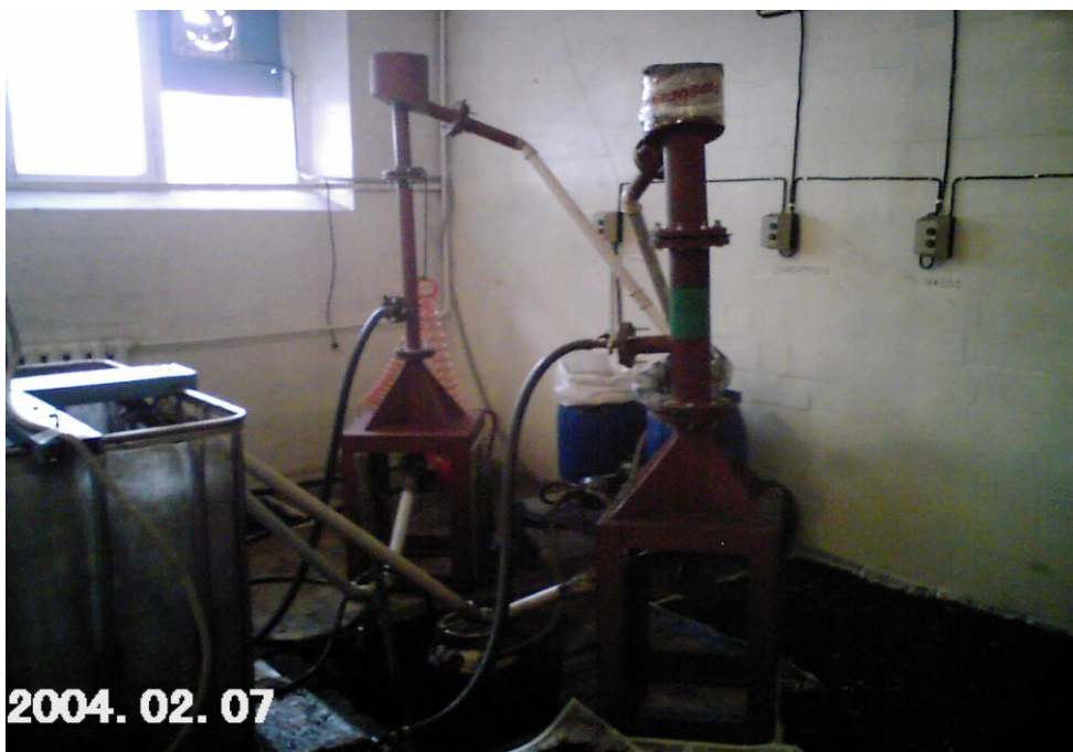
Figure 40 – A photography of the columns of the main and cleaner flotation
